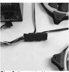
**Step 3**: Connect the Molex 4 pin connectors to the power supply
