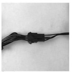
**Step 1**: Connect the light effect sync cable from the main fan and all sub fans
