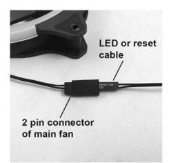
**Step 2**: Connect 2 pin connector of the main fan to the LED or reset cable of the chassis
